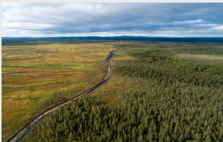
The waterline at Kittilä mine will facilitate water management at the site by allowing a greater discharge rate while maintaining water quality and meeting all environmental regulations.
