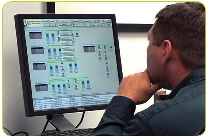
Today, engineers enjoy end-to-end control of plant processes. The easy-to-learn graphical interface enables employees in the operating center to see a real-time representation of the capacity of water moving through the facility, plus they can control the process and monitor error and fault codes from all of the PLCs. And when they leave the operating center, SCADA terminals throughout the plant enable access to the Wonderware system wherever they may be working.
